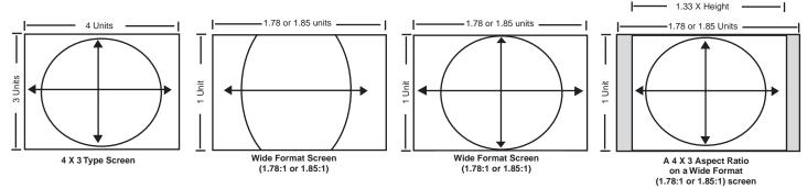
**4 X 3** - Use horizontal size to make image fit width of screen, then use vertical size to make image fill height (circle is round). On a wide format (1:78:1 or 1.85) screen, adjust width of image 1.33 X the height of the screen. Adjust the vertical size to fill the height.
